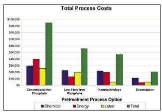
Zirconization reduces chemical, energy, and maintenance costs compared to other pretreatment processes.
