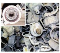
Zirconization reduces sludge and scale build-up typical of conventional iron phosphate process.
