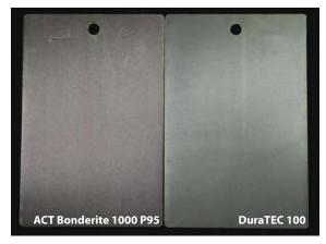
Both conventional iron phosphate and the Zirconization Process produce an even blue, purple, or gold coating depending on the process parameters.
