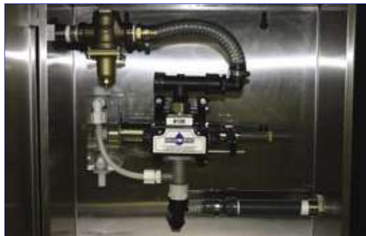
Coolant mixing system for precision concentration control.
