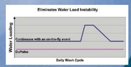
The DuPulse method does not add water to the press felts as other methods do.
